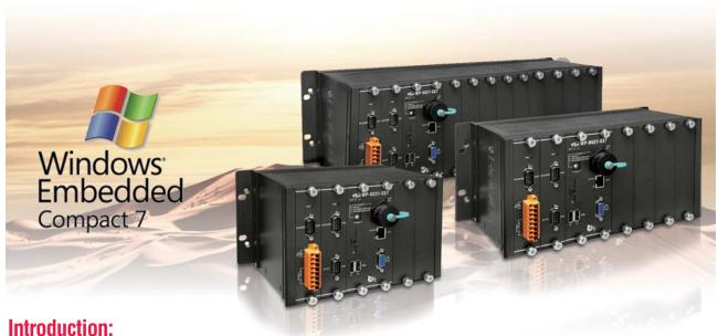
The WP-9000 is a compact (3U), rugged PAC. It provides Cortex-A8 ARM CPU, dual gigabit ethernet, two USB ports, VGA ports, SD card slot and redundant power input. It is a upgrade version of WP-8000. Moreover, WP-9000 can be widely used in Factory Automation, Building Automation, Machine Automation, Laboratory Automation, Chemical industry, environmental monitoring, M2M, IIOT, Industrial 4.0 ...etc
