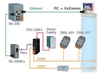
Because of these reasons, optical fibers have largely replaced copper wire communications in core networks in the developed world. The user-friendly VxComm Driver/Utility allows users to easily turn the built-in COM ports of the PDS-220Fx series into standard COM ports on a PC. By virtue of its protocol independence, a small-core OS and high flexibility, the PDS-220Fx series is able to meet the demands of every network-enabled application.
