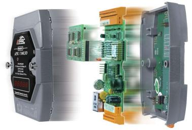
in one X-Board. The X-Board allows users to implement various I/O functions such as DI, DO, A/D, D/A, Timer/Counter, UART, flash memory, battery backup SRAM, AsicKey & other I/O functions.
