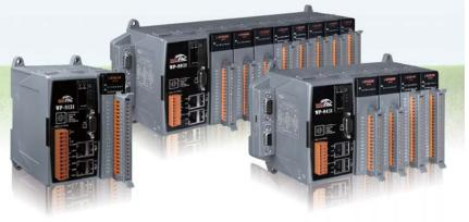
WinPAC-8000 is the new generation PAC of ICP DAS. It is equipped a ARM CPU running a Windows CE.NET operating system, various connectivities (VGA, USB, Ethernet, RS-232/485) and 1/4/8 slots for high performance Parallel I/O modules (high profile I-8K series) and serial I/O modules (high profile I-87K I/O modules).
