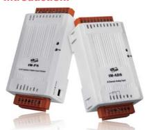
The tM series is a family of network data acquisition and control modules with digital or analog I/O functions. The modules can be remotely controlled through an RS-485 serial bus by using DCON and Modbus RTU/ASCII protocols. The selectable transmission speed of the RS-485 port is up to 115,200 bps. Modbus has facto standard communications protocol in industry, and is now the most commonly available means of connecting industrial electronic devices.
