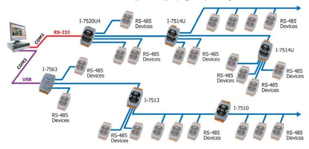
The following block diagram shows how I-7514U was designed as independent channel. Data coming from the master input will be transmitted to all four RS-485 slave channels. But data coming from the slave channels will be returned to the master input only. Thus reduces the possibility of interference between each RS-485 slave loop and makes the RS-485 networks more robust and reliable.
