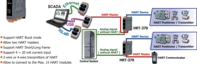
Support the in point-to-point or multi-drop HART network
